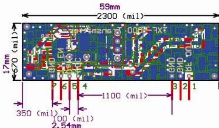
TXF-1000U Transmitter board size keepout
